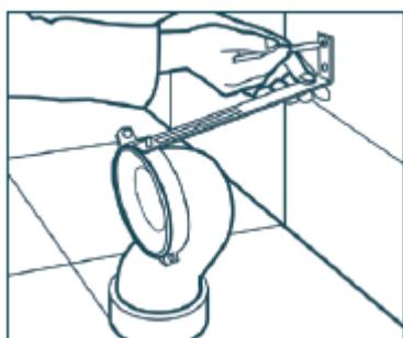
„S“ bend is mounted to its place and attached to the wall with the metal sheet bar.
