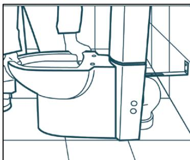
After connecting the cistern, connect the monobloc to the drainage pipe
