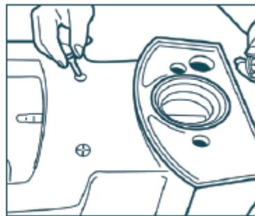
Screws for Cistern and toilet seat are mounted and water leakage test is performed.
