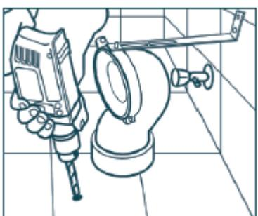
Holes are drilled with a suitable drill and fixing plugs are driven. Plastic mounting component is mounted on the floor.
