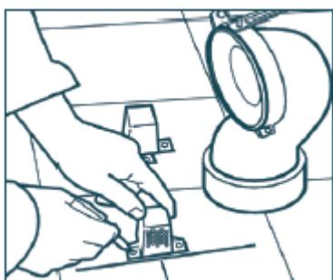
Toilet is removed from its place and puller mounting component is put on the floor in a way to center the hole axis.
