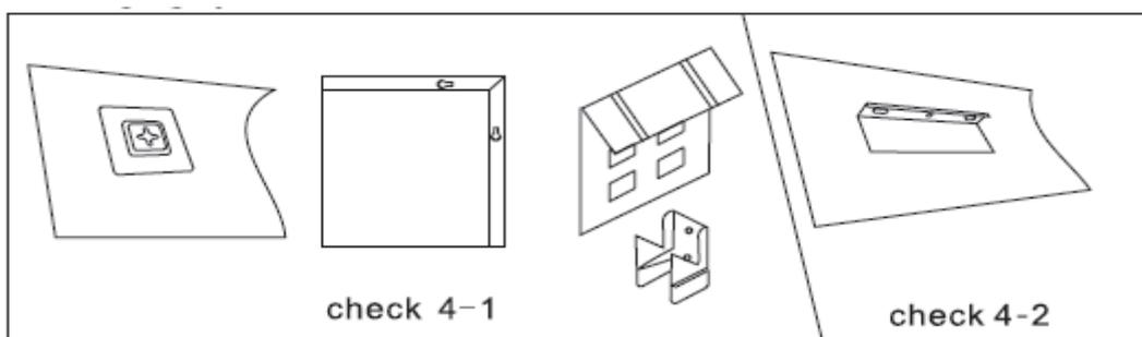
2. Measure the distance between two brackets, install the expansion bolt and screw on the wall.
