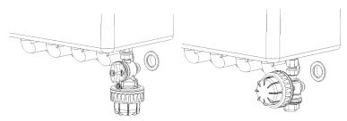
The polyphosphate doser is to be installed on the domestic cold water line at the boiler inlet.
