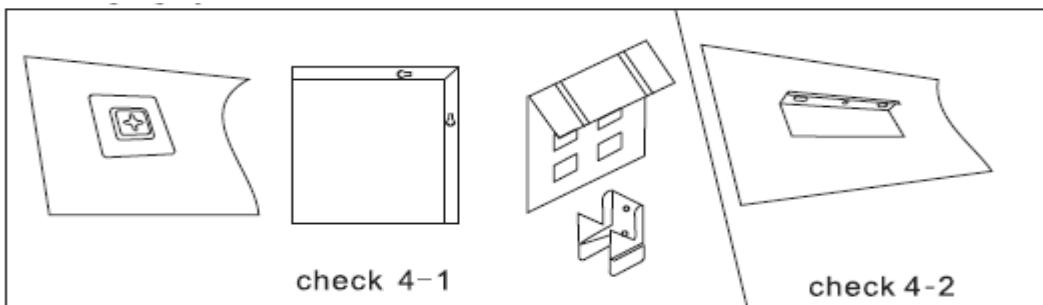
**2.** Measure the distance between two brackets, install the expansion bolt and screw on the wall.
