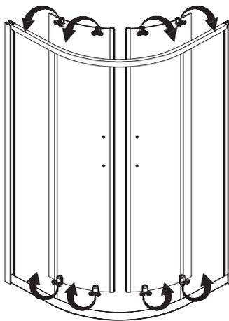
**5** Hang the top rollers onto the top track, press the buttons of the bottom rollers to put them into the bottom track.
