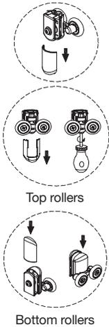
When fitting the top rollers, make sure the wheel adjuster screw is facing down the length of the glass door facilitate correct wheel alignment.
