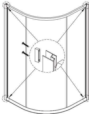
**1** Fit plugs (10) to the two ends of connection profiles. Fix the connection profile (4) and 2 tracks using M4\*30 round screws to form a frame.
