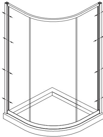
**4** Fix the wall profiles to wall using M4\*30 screws. Cover screws with capped washers. Push the frame to wall profiles.
