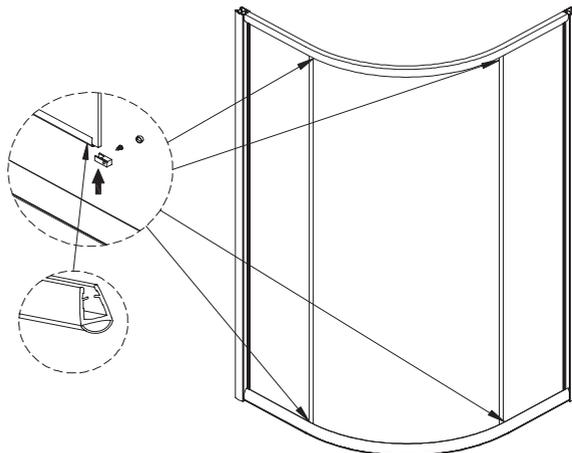
**2** Fit glass clips to the fixed glass panel, fasten fixed panel to track by tightening the screws of glass clips into the track hole. Cover screws with screw caps.
