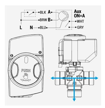
The actuator can be moved manually by pushing and rotating the knob to the desired position.
