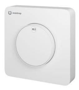
The ClimaCon F room thermostats are used to control the temperature of surface heating and cooling systems as well as heating and cooling ceilings in detached houses or flats. The room temperature is controlled via a valve, which is controlled by the room thermostat via an electrothermal actuator. When the room temperature reaches the target temperature, the valve is closed.
