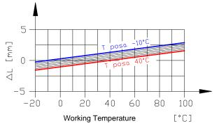
The diagram on the side shows the linear expansion of 1 m of pipe (measured at a "T  $_{\text{Laying}}$ ") as soon as the pipe is put into operation.
