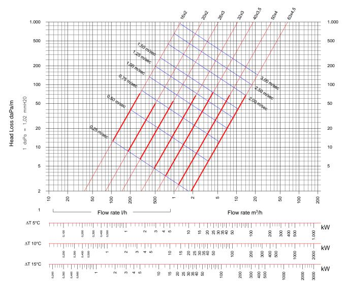
The graph shows the pressure drop as a function of the fluid flow rate in l/h or in  $m^3/h$  or as a function of the system potential in KW (please use the scale suitable for the  $\Delta T$  temperature gradient of the water).
