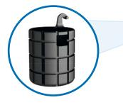
Optimised float geometry for minimum capillary effect – avoids the formation of an air cushion to suppress undefined "jumps" of the float.
