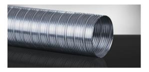
**Texoflex AL** s made of single layer corrugated aluminium AL 99,5 resistant to moisture. Due to transport and dimensional stability the duct can be compressed to approx. 1/3 of its length.
