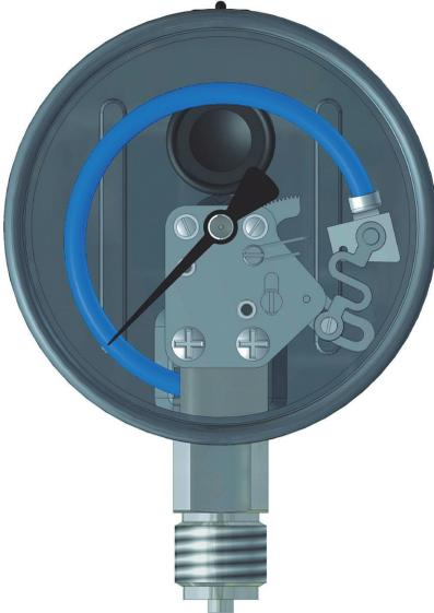
The products contain measuring elements (Bourdon tubes) which are deformed if pressure is applied. This motion is transmitted to a movement.
