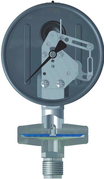
Diaphragm pressure gauges use circular corrugated diaphragms. The pressure to be measured is applied at one side. The deflection of the diaphragm is proportional to the pressure.
